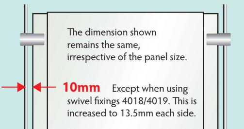
When using 6mm rod, the distance between the rod centre and the edge of the panel should be 10mm.
