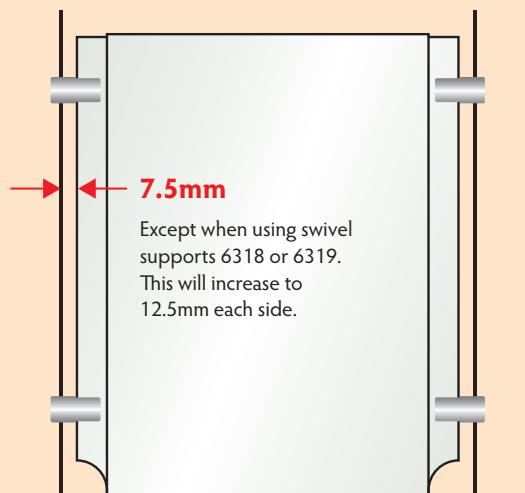
When using 3mm cable, the distance between the cable centre and the edge of the panel should be 7.5mm.
